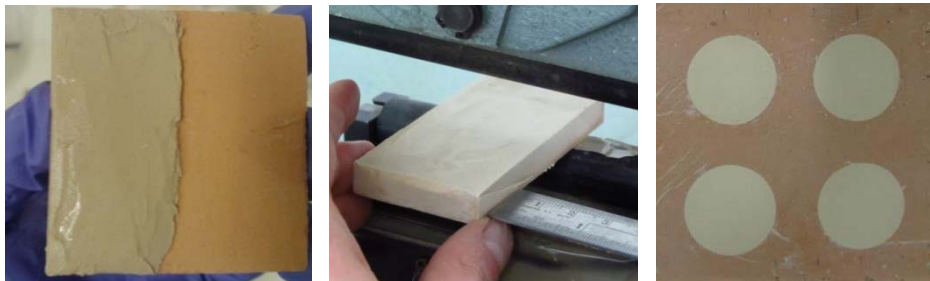
Figure 2. Geopolymer pastes and examples of some tests performed to characterize them. a) Visual observation of the pastes, b) Mechanical strength test (bending), and c) Samples for adhesion strength test (pull-off). Photos by C. Geraldes.
